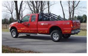
The X-Tra-Lift has numerous options available. An optional remote control key fob is available with a range of 200-feet. A variety of carriers are available with a steel, aluminum or open deck. A personal water craft carrier is also available. Many light packages are also offered to mount on the top bar of the X-Tra-Lift.
